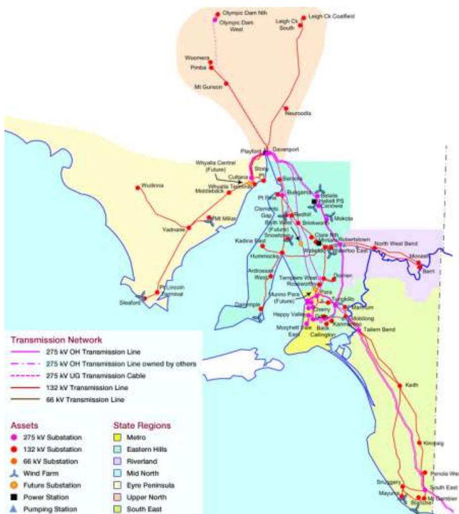
Figure14: South Australia Electricity Transmission System (source: Electranet)
